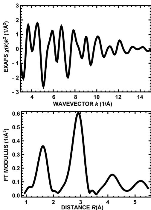
**Figure 1** Experimental Zn K-edge EXAFS spectrum  $\chi(k)k^2$  and its Fourier transform (FT) for polycrystalline ZnO measured at room temperature.
