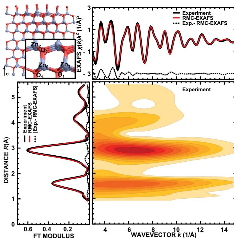
**Figure 3** Supercell used in the RMC simulation (blue large balls are zinc atoms, red small balls are oxygen atoms) (upper left panel), the experimental and calculated (corresponding to the final RMC configuration) Zn K-edge EXAFS spectra and their difference (upper right panel), Fourier transforms of the experimental and calculated EXAFS spectra and their difference (bottom left panel), and the Morlet wavelet transform of the experimental EXAFS spectrum (bottom right panel).
