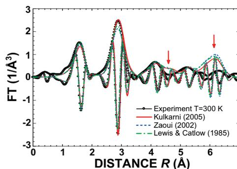
**Figure 2** Fourier transforms of the experimental and MD-EXAFS Zn K-edge EXAFS spectra. The MD-EXAFS spectra were calculated using three different force-field models [23–25].
