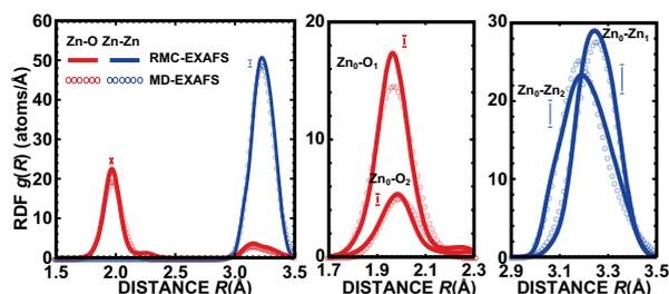
**Figure 4** Radial distribution functions (RDFs) of oxygen (red lines) and zinc (blue lines) atoms around absorbing zinc atom, obtained from the MD simulations with the force-field model by Kulkarni [23] (circles) and from the RMC/EA-EXAFS analysis (solid lines): total RDFs (left panel) and partial RDFs corresponding to non-equivalent oxygen (middle panel) and zinc atoms (right panel). The vertical bars indicate the estimated maximal uncertainties.
