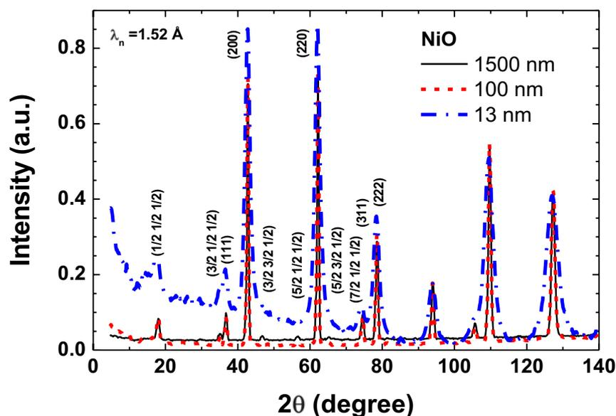
Fig. 1. Neutron diffraction pattern for NiO powders at room temperature.
