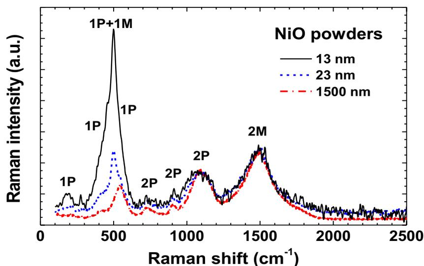
Fig. 2. Room temperature micro-Raman spectra of the NiO powders having grain size 13, 23 and 1500 nm.
