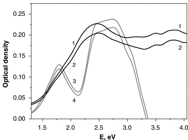
Fig. 1. The spectra of the transient optical density induced by electrons in the MgO single crystals, preliminary irradiated by the fast neutrons: (1) fluence  $10^{16}$  cm<sup>-2</sup>, 20 ns delay after start of the excitation pulse; (2) fluence  $10^{16}$  cm<sup>-2</sup>, 5000 ns delay; (3) fluence  $10^{18}$  cm<sup>-2</sup>, 20 ns delay after start of the excitation pulse; (4) fluence  $10^{18}$  cm<sup>-2</sup>, 5000 ns delay.
