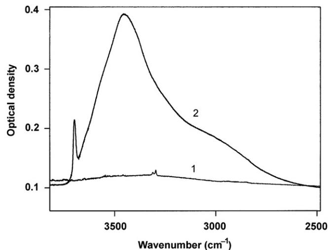
Fig. 2. The infrared absorption spectra of the MgO crystal irradiated by the fast neutrons: (1) fluence  $\Phi = 10^{16}$  cm<sup>-2</sup> and (2)  $\Phi = 10^{18}$  cm<sup>-2</sup>.
