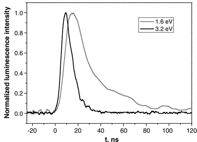
Fig. 4. The luminescence decay kinetics for different emission bands of the MgO crystal (fluence  $10^{16} \text{ cm}^{-2}$ ).
