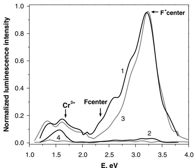
Fig. 3. The spectra of luminescence excited by the pulsed electron beam in the MgO single crystals, preliminary irradiated by the fast neutrons: (1) fluence  $10^{16} \text{ cm}^{-2}$ , 20 ns delay after start of the excitation pulse; (2) fluence  $10^{16} \text{ cm}^{-2}$ , 100 ns delay; (3) fluence  $10^{18} \text{ cm}^{-2}$ , 20 ns delay after start of the excitation pulse; (4) fluence  $10^{18} \text{ cm}^{-2}$ , 100 ns delay.
