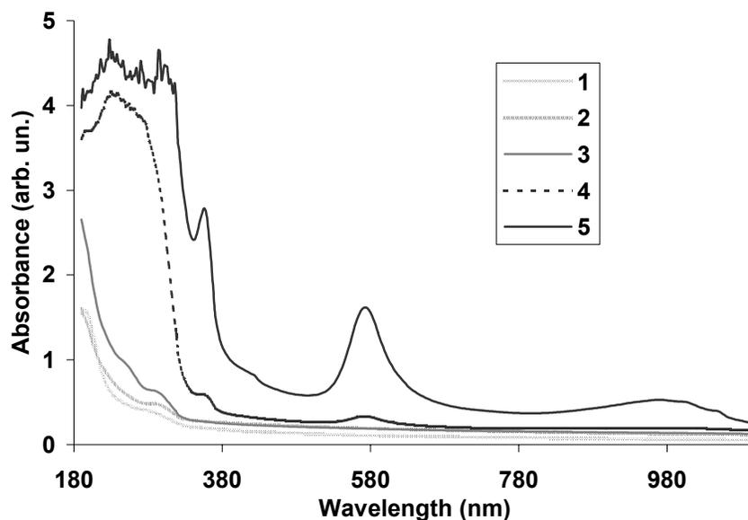
Fig. 1. Optical absorption spectra of MgO (III) crystal: 1 - before irradiation; after fast neutron irradiation with 2 -  $\Phi = 10^{14} \text{ cm}^{-2}$ , 3 -  $\Phi = 10^{15} \text{ cm}^{-2}$ , 4 -  $\Phi = 10^{16} \text{ cm}^{-2}$ , 5 -  $\Phi = 10^{18} \text{ cm}^{-2}$ .
