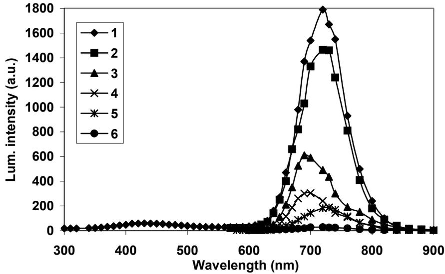
Fig.4. Photoluminescence spectra of MgO (I): 1 - nonirradiated,  $\lambda_{ex}=214$  nm, 2 - nonirradiated,  $\lambda_{ex}=420$  nm, 3-6. irradiated by fast neutron fluence,  $\lambda_{ex}=214$  nm, 3 -  $\Phi=10^{14}$  cm<sup>-2</sup>, 4 -  $\Phi=10^{15}$  cm<sup>-2</sup>, 5 -  $\Phi=10^{16}$  cm<sup>-2</sup>, 6 -  $\Phi=10^{18}$  cm<sup>-2</sup>.
