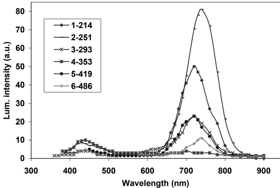
Fig.6. Photoluminescence spectra of MgO (II) crystal irradiated by fast neutrons with fluence  $\Phi=10^{15} \text{ cm}^{-2}$  at different excitation wavelengths.
