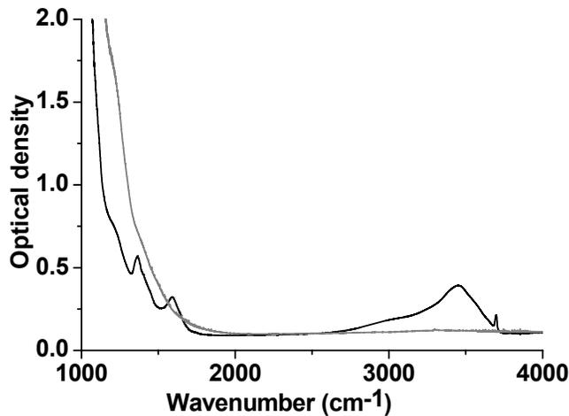
Fig. 7. Infrared absorption spectra of MgO crystal irradiated by fast neutrons: grey line - fluence  $\Phi=10^{16} \text{ cm}^{-2}$ , black line -  $\Phi=10^{18} \text{ cm}^{-2}$ .
