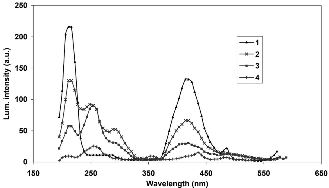
Fig.3. Photoluminescence excitation spectra of MgO (II) crystals: 1 - nonirradiated, 2 - irradiated by fast neutron fluence  $\Phi=10^{14}$  cm<sup>-2</sup>, 3 -  $\Phi=10^{15}$  cm<sup>-2</sup>, 4 -  $\Phi=10^{16}$  cm<sup>-2</sup>.
