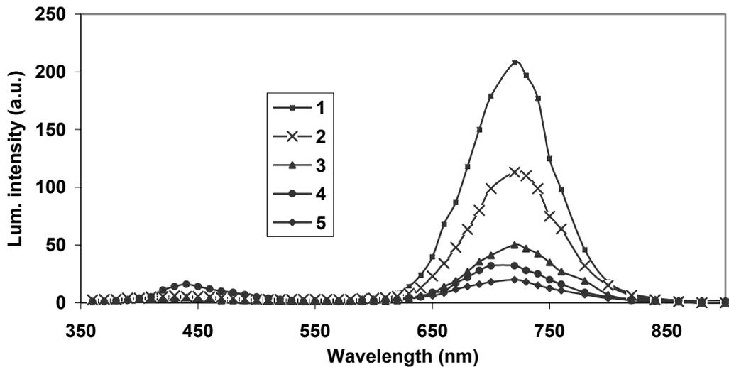
Fig.5. Photoluminescence spectra of MgO (II)  $\lambda_{ex}=214$  nm: 1 - nonirradiated; irradiated by fast neutron fluence 2 -  $\Phi=10^{14}$  cm<sup>-2</sup>, 3 -  $\Phi=10^{15}$  cm<sup>-2</sup>, 4 -  $\Phi=10^{16}$  cm<sup>-2</sup>, 5 -  $\Phi=10^{18}$  cm<sup>-2</sup>.
