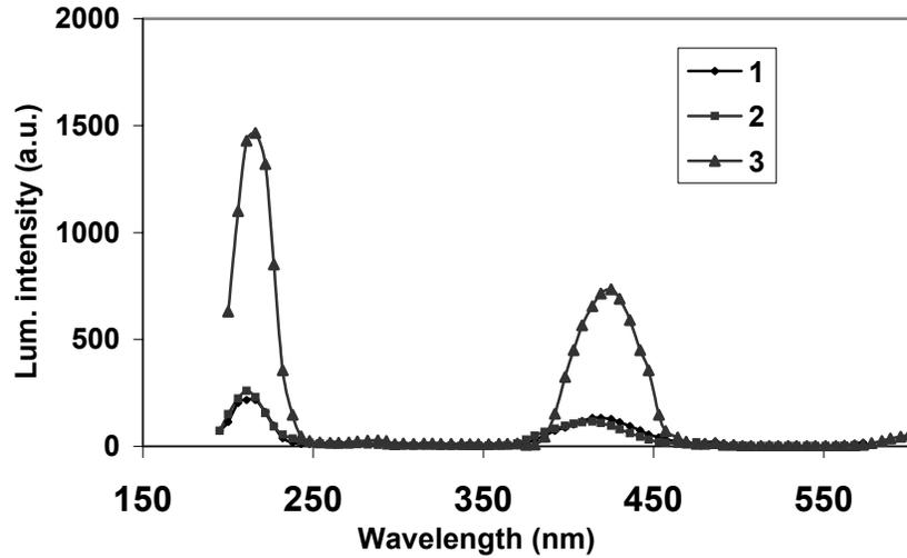
Fig.2. Photoluminescence excitation spectra of nonirradiated crystals: 1 - MgO (II), 2 - MgO (I), 3 - MgO (III) ( $\lambda_{lum} = 730$  nm).
